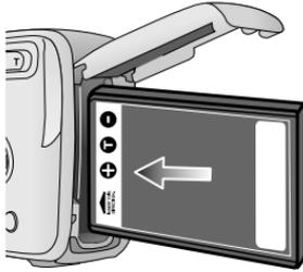
2. Insert the batteries taking note of the polarity (+ / -).
